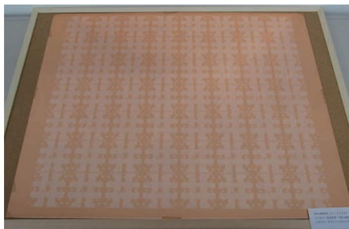
FPA-8000iW Steppers have demonstrated submicron resolution on panel substrates
